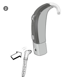
2 Close the battery door again and plug in the cable as shown
